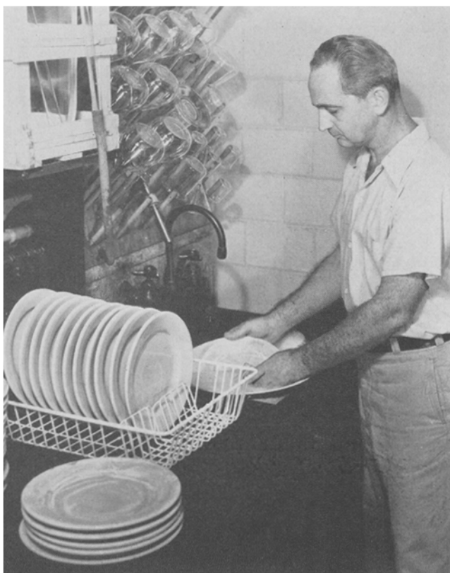
Fig. 4. Semipractical plate wash test.
